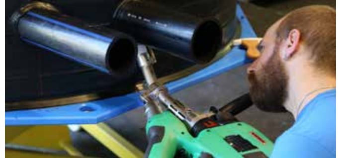
Unattainable is weldable with the new 45° and 90° angled adapters.
