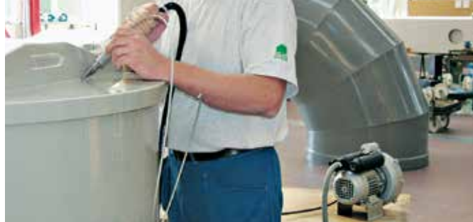
ROBUST blower, serving as the external air supply for the WELDING PEN.
