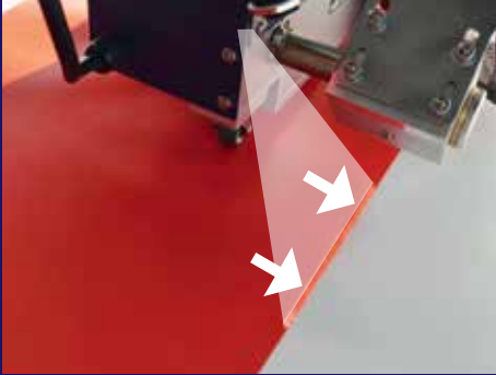
Laser guide for more accuracy
