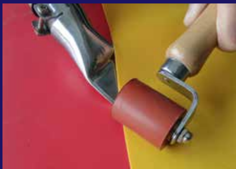
The suggested Weldy hot air hand tools for tarpaulins and billboards
