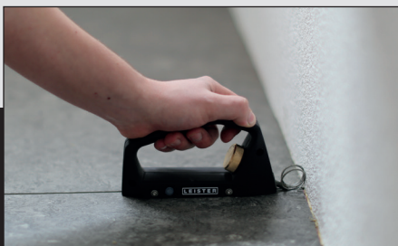
Executing clean grooves up to connecting walls
